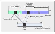
Establishing fast data exchange between kernel-space and user-space: a page frame to host the monitored memory is kmalloc'ed in kernel-space, in the conte. of a special char device ("kmem\_mapper"). When the device is mmap'ed in the user program, the page is remapped to user-space and can be directly accessed. The "mwmon\_mmap\_area" pointer in kernel-space, and the "mmapped\_dev\_-mem" pointer in user-space, both point to the beginning of the monitored region.
