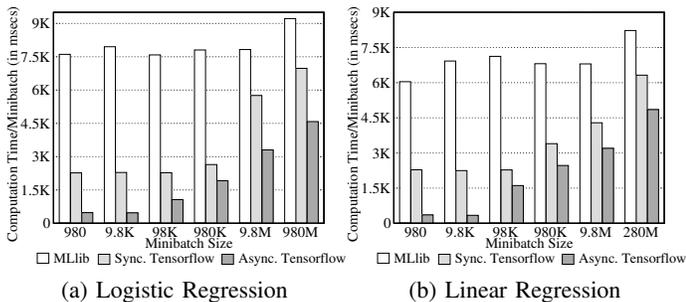
Fig. 3: Computation time per minibatch in MLib and TensorFlow (synchronous and asynchronous) on a 141-node cluster.
